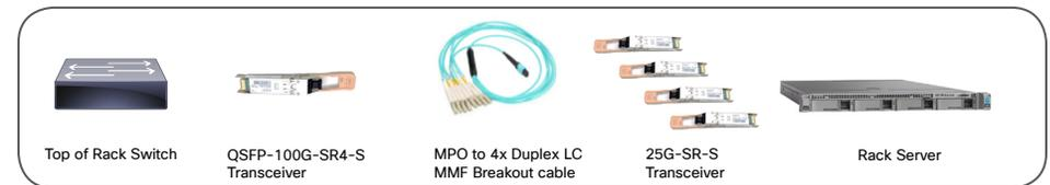
Cisco's SFP-10/25G-CSR-S transceivers can be used with Cisco's QSFP-40G-SR4-S and Cisco's QSFP-100G-SR4-S using 3<sup>rd</sup> party MMF break-out cables.\*, #
